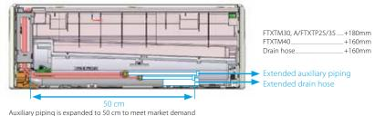
Auxiliary piping is expanded to 50 cm to meet market demand and decrease installation time. It's also adapted to fit the wall thickness of Scandinavian houses.
